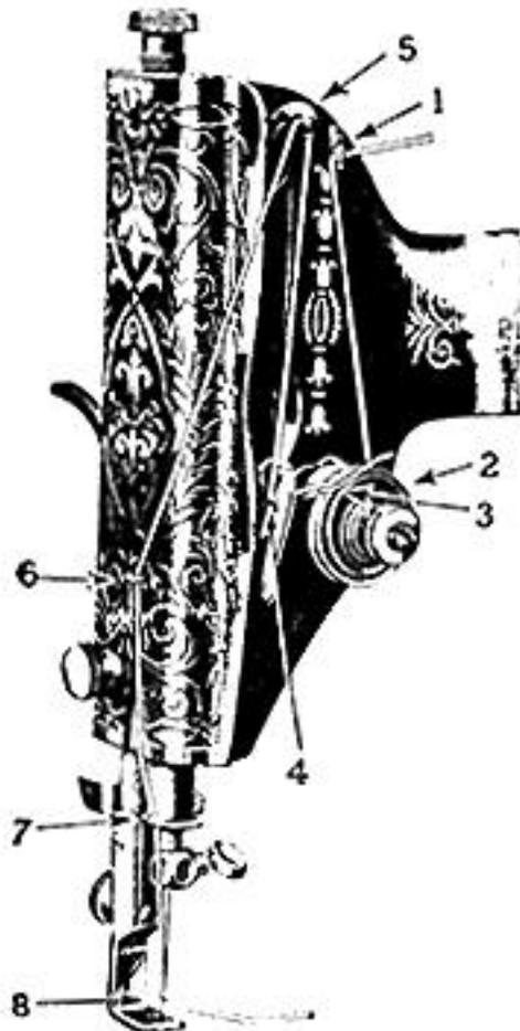
FIG. 11. THREADING THE NEEDLE
