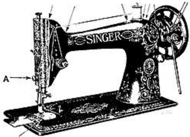
FIG. 17. FRONT VIEW, SHOWING OILING POINTS
